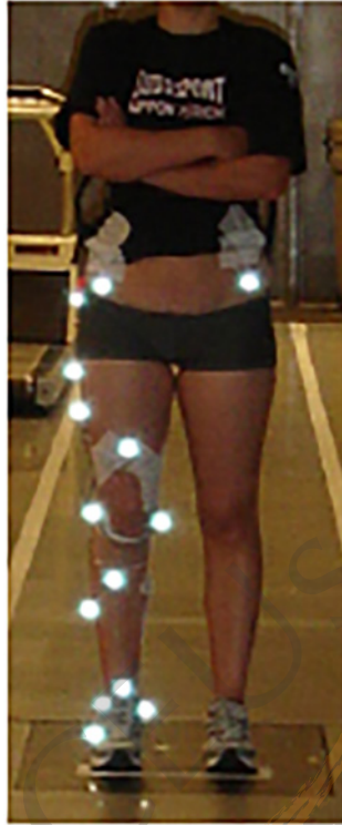
Fig 1. Marker Set Up. Frontal view of retro-reflective marker placement on the shoe, shank, thigh and pelvis.
